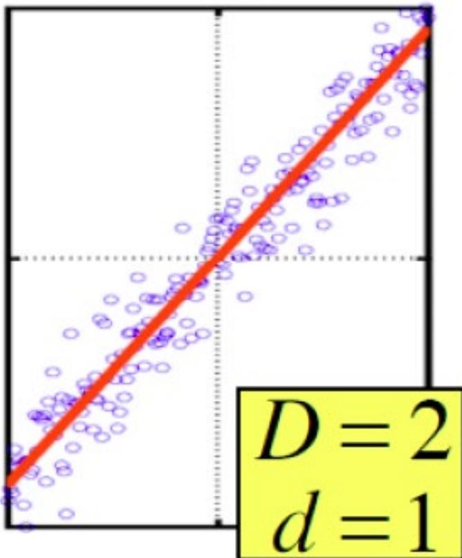
Rather than representing every point with 2 coordinates we represent each point with 1 coordinate (corresponding to the position of the point on the red line).
